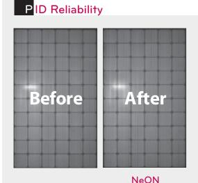
The NeON cell is a high-efficiency module compared to the standard mono-crystalline cell structure and has better PID\* rating than many other modules. The NeON passed the Frauenhofer CSP PID\* test. This means the NeON panels are well equipped to withstand high voltage stress. \*PID (Potential Induced Degradation)
